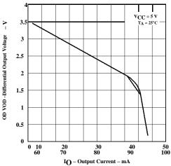
Figure 10. Driver Differential Output Voltage vs
