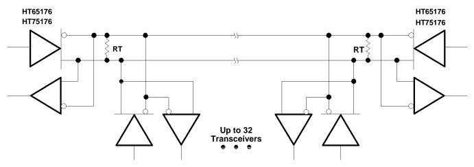
The line should be terminated at both ends in its characteristic impedance ( $R_T = Z_O$ ). Stub lengths off the main line should be kept as short as possible.
