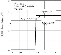
V<sub>I</sub> – Enable Voltage – V Figure 15. Receiver Output Voltage VS Enable Voltage
