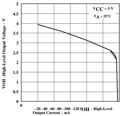
Figure 8. Driver High-Level Output Voltage vs
