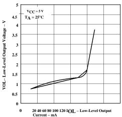
Figure 9. Driver Low-Level Output Voltage
