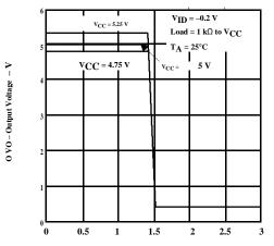
$\begin{array}{c} v_{I} - {\rm Enable\ Voltage} - v \\ \text{Figure\ 16.\ Receiver\ Output\ Voltage} \\ vs \\ \text{Enable\ Voltage} \end{array}$
