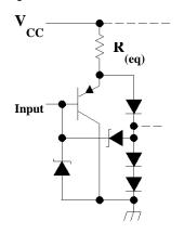
Driver input:  $R(eq) = 3 \text{ k}\Omega \text{ NOM}$ Enable inputs:  $R(eq) = 8 \text{ k}\Omega \text{ NOM}$
