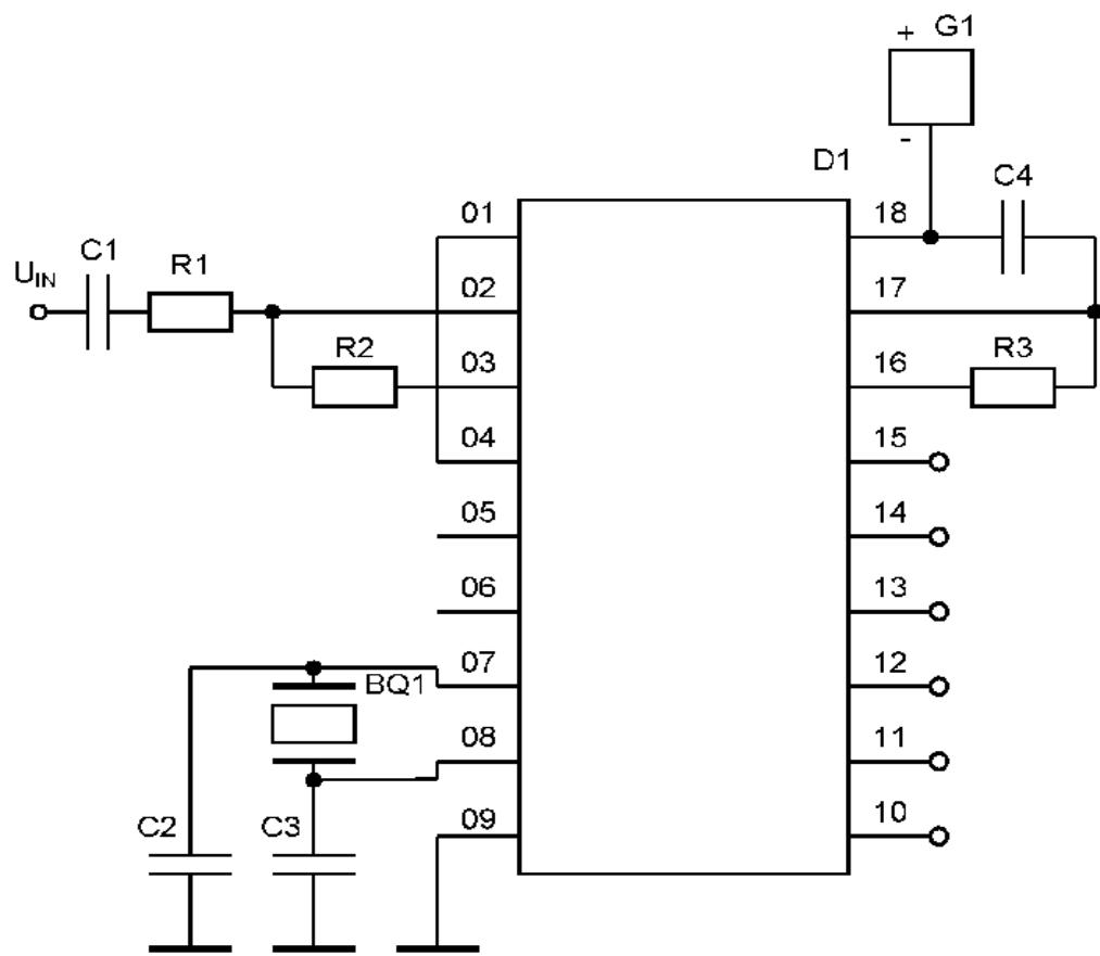
BQ1 – quartz resonator with frequency 3,579545 MHz
