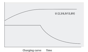
For the charging itself it is not important if the battery is partly or completely discharged. The battery can stay connected to the charger for a long period, the surrounding temperature should be in the range of 10°C to 25°C. In case the battery has been connected to the charger with the wrong polarity then this will be indicated through a red light (**"verpolt"**). Disconnect the battery from the charger immediately.
