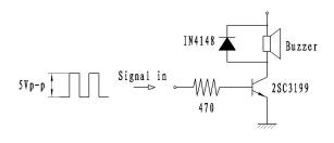
Resonant frequency, 1/2 duty cycle. Square wave. Signal amplitude should be large enough tosaturate the transistor.
