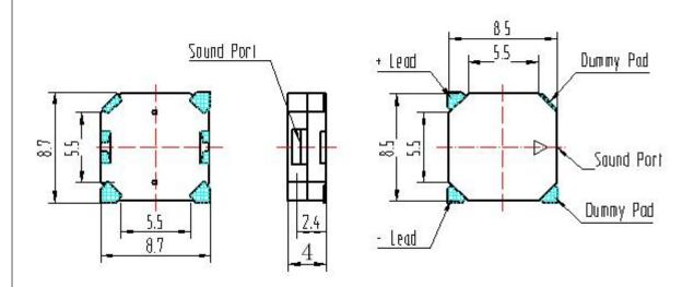
\*Unit: mm; Tolerance: ± 0.3mm Except Specified
