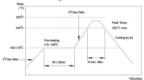
Note: (1) In automated mounting of the SMD sound transducers on PCB, any bending, expanding and pulling forces or shocks against the SMD sound transducers shall be kept minimum to prevent them from electrical failures and mechanical damages of the devices.(2) In the reflow soldering, too high soldering temperatures and too large temperature Gradient such as rapid heating or cooling may cause electrical failures and mechanical
