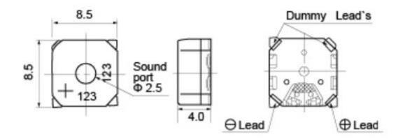
\*Unit: mm; Tolerance: ± 0.3mm Except Specified \*Housing Material: Black LCP \*Terminal plate: 3 soldering pads, tin Plating Brass
