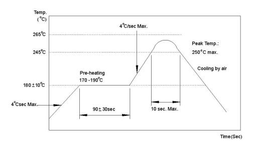
Note: (1) In automated mounting of the SMD sound transducers on PCB, any bending, expanding and pulling forces or shocks against the SMD sound transducers shall be kept minimum to prevent them from electrical failures and mechanical damages of the devices. (2) In the reflow soldering, too high soldering temperatures and too large temperature Gradient such as rapid heating or cooling may cause electrical failures and mechanical damages of the devices.
