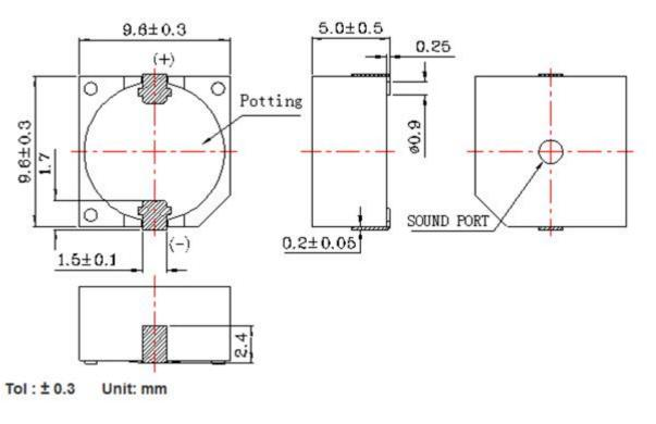
\*Unit: mm; Tolerance: ± 0.3mm Except Specified \*Housing Material: Black LCP \*Terminal plate: 2 soldering pads, tin Plating Brass
