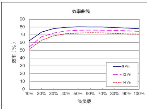
效率曲线 ( $V_{out}=0.7V$ )
