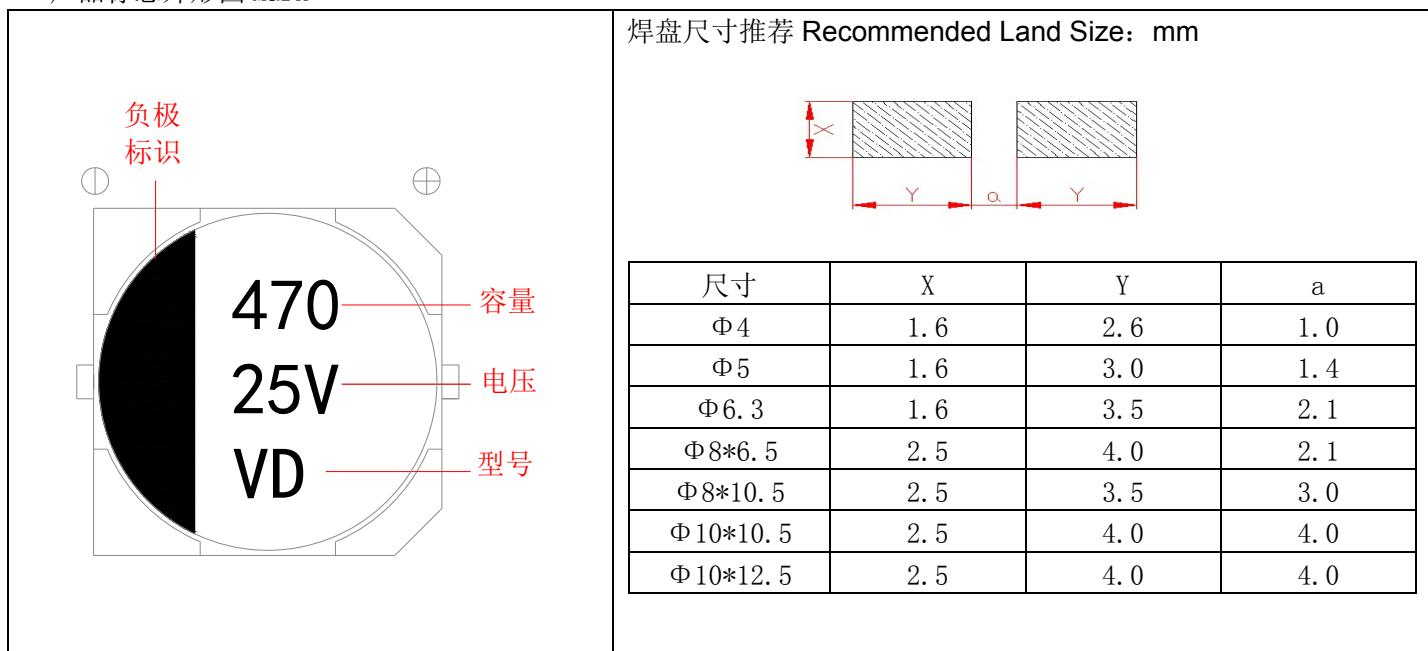
The diagram shows a circular capacitor with markings: '负极标识' (negative terminal indicator) at the top left, '容量' (Capacity) with '470' at the top right, '电压' (Voltage) with '25V' at the bottom right, and '型号' (Model) with 'VD' at the bottom left. To the right is a table titled '焊盘尺寸推荐 Recommended Land Size: mm' showing dimensions X, Y, and a for various case sizes.
