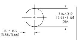
PANEL CUT OUT HUBER+SUHNER Astrolab REFERENCE "PC4" TORQUE MOUNTING NUT TO 20±2 IN-LBS [2.96±.3 Nm]
