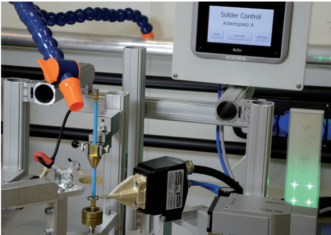
Temperature controlled soldering
