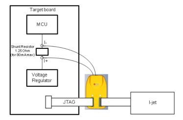
This figure shows how I-scope is connected to I-jet Trace and to the target board:
