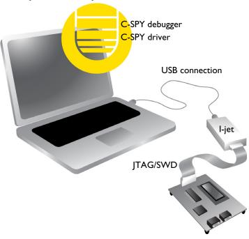
I-jet communicates using USB 2.0. USB 1.0 is also supported but not advised. The I-jet in-circuit debugging probe is also referred to as a debug probe, debug adapter, or JTAG in-circuit emulator by different tool vendors.
