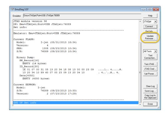
**3** In the dialog box that is displayed, browse to the arm\bin\jet\firmware\i-jet folder of your IAR Embedded Workbench installation. In one of the subfolders, select the firmware file that you want to use and click **Open**.
