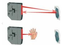
interrupts the beam) so Excess Gain is reduced and maximum operating distances can reach 12 meters. It is necessary to operate in clean environments without dirt or dust. A retro-reflective sensor typically operates in the dark mode: output is activated when an object interrupts the light beam between the sensor and reflector.
