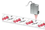
green. For general purposes a white light is used because the full light spectrum detects the majority of contrasts. White light emission is obtained through lamps, or LEDs in most sensors, enabling the detection of very slight contrasts due to different surface treatments, even of the same material and color.
