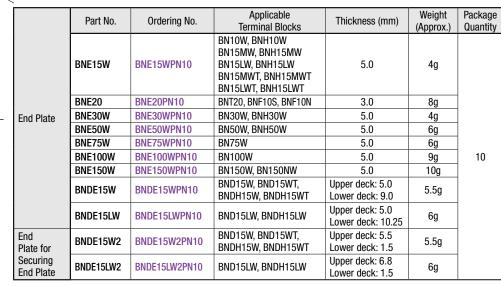
Note: BNDE15W2 and BNDE15LW2 are end plates used for securing marking strips at the end of double deck terminal blocks.
