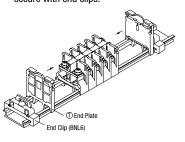
3. Insert the marking strip holder into the recess of the end plate.
