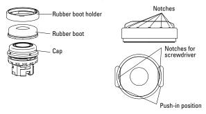
Push the rubber boot holder further around on the two notches on the holder so that the holder fits the button completely
