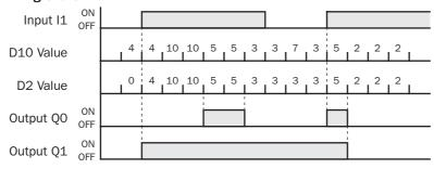
Output Q0 is on when data register D2 value is 5.
