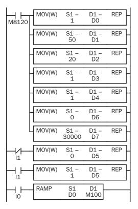
M8120 is the initialize pulse special internal relay.
