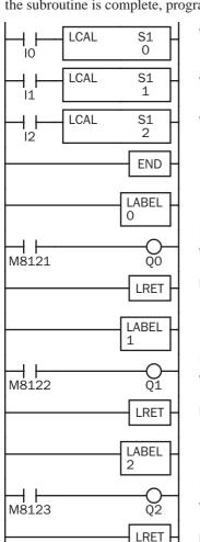
When input IO is on, program execution jumps to label 0.
