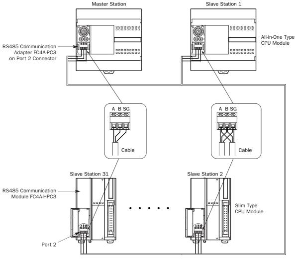
Shielded twisted pair cable 200 meters (656 feet) maximum Core wire  $0.3 \mathrm{mm}^2$
