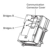
**1.** Carefully push in the communication connector cover at position (1) to break bridges A as shown in either figure below.
