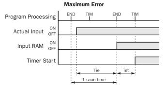
When the input turns on immediately after the END processing, Tie is almost equal to one scan time. Then the timer input error is Tie + Tet = one scan time + Tet (behind error) and is at its maximum.
