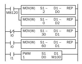
M8120 is the initialize pulse special internal relay.
