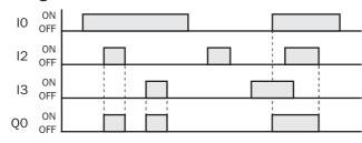
When input IO is on and either input I2 or I3 is on, output Q0 is on.
