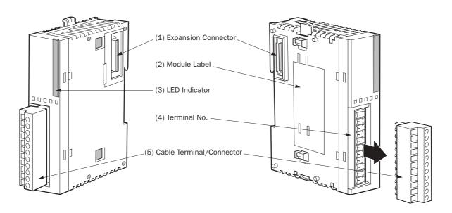
The above figures illustrate the 8-point relay output module.
