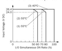
When using at 40°C, all I/Os can be turned on simultaneously at 26.4V DC as indicated with line (3).
