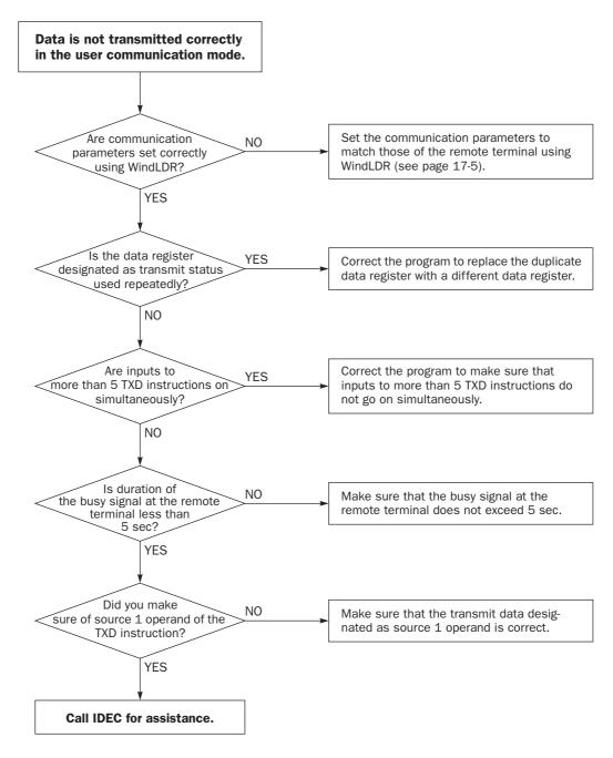
When the user communication still has a problem after completing the above procedure, also perform the procedure of Diagram 9 described on the preceding page.
