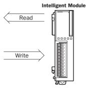
While the CPU module is running and the input is on, RUNA READ is executed to read data from the intelligent module, and RUNA WRITE to write data to the intelligent module.
