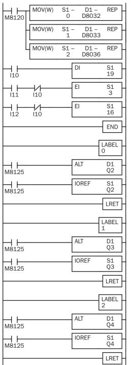
M8120 is the initialize pulse special internal relay.
