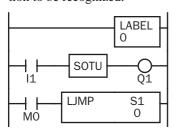
Although normally, the SOTU instruction produces a pulse for one scan, when used in a program branch the SOTU pulse will last only until the next time the same SOTU instruction is executed.
