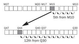
As a result, when input IO is on, the ON/OFF status of internal relay M15 is moved to output Q44.
