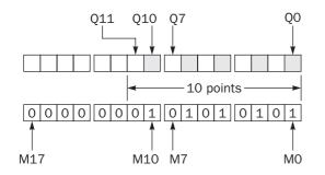
This program will invert the status of the shaded outputs at the left from on to off, and those not shaded from off to on.
