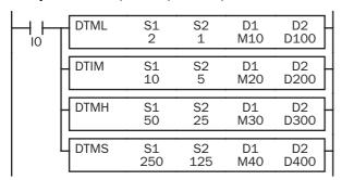
While input IO is on, four dual timer instructions turn on and off the destination operands according to the on and off durations designated by source operands S1 and S2.
