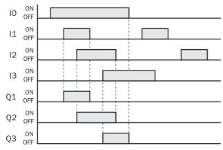
When both inputs IO and I1 are on, output Q1 is turned on.
