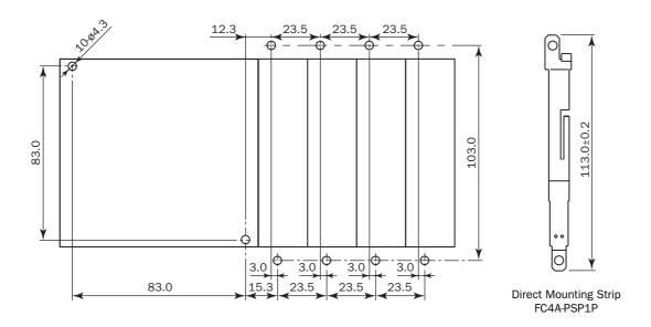
Example 2: Mounting hole layout for, from left, FC4A-HPH1, FC4A-D20K3, FC4A-N16B3, FC4A-N32B3, and FC4A-M24R2 modules
