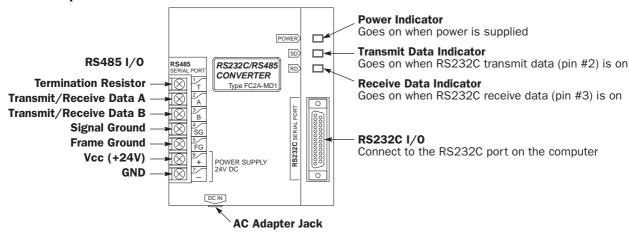
**Note:** Connect 24V DC to POWER SUPPLY + and – terminals or connect an AC adapter with 9V DC, 350mA output to the AC adapter jack.
