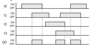
When both inputs IO and I1 are on or both inputs I2 and I3 are on, output Q0 is on.
