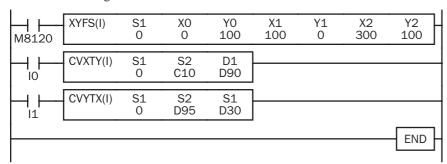
M8120 is the initialize pulse special internal relay.
