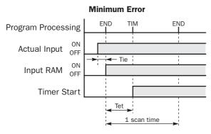
When the input turns on immediately before the END processing, Tie is almost 0. Then the timer input error is only Tet (behind error) and is at its minimum.
