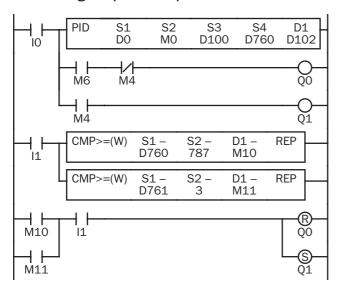
While input IO is on, the PID instruction is executed.
