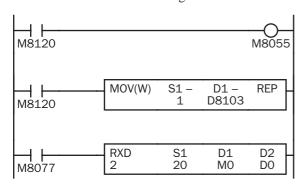
M8120 is the initialize pulse special internal relay.
