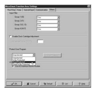
3. Under Protect User Program, select a required protect mode in the pull-down list.
