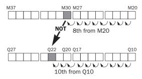
As a result, when input IO is on, the ON/OFF status of internal relay M30 is inverted and moved to output Q22.
