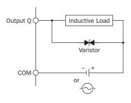
This protection circuit can be used for both AC and DC load power circuits.
