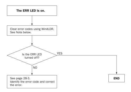
**Note:** Temporary errors can be cleared to restore normal operation by clearing error codes from WindLDR. See page 28-2.
