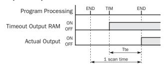
Timeout output error is equal to Tte (behind error) and can be between 0 and one scan time.
