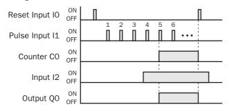
• The preset value 0 through 65535 can be designated using a data register D0 through D1299 or D2000 through D7999; then the data of the data register becomes the preset value. Directly after the CNT instruction, the OUT, OUTN, SET, RST, TML, TIM, TMH, or TMS instruction can be programmed.
