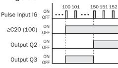
Output Q3 is on when counter C20 current value is between 100 and 149.
