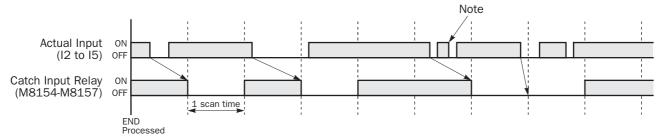
Note: When two or more pulses enter within one scan, subsequent pulses are ignored.
