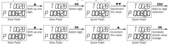
**5.** The changed preset value is displayed without flashing. Write the new preset value to the CPU module RAM.
