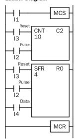
When input I1 is on, the MCS is not executed so that the counter and shift register are executed according to actual statuses of subsequent inputs I2 through I4.
