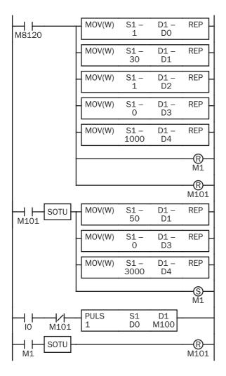
M8120 is the initialize pulse special internal relay.
