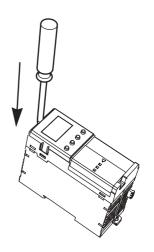
**2.** While turning the screwdriver in the direction as shown, disengage the latch on the HMI module and pull out the HMI module.
