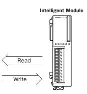
When the CPU module is stopped, STPA READ is executed to read data from the intelligent module, and STPA WRITE to write data to the intelligent module.
