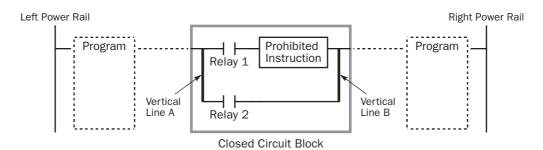
The error detection depends on the version of WindLDR. When using WindLDR ver. 4.4 or earlier, particular care is needed.
