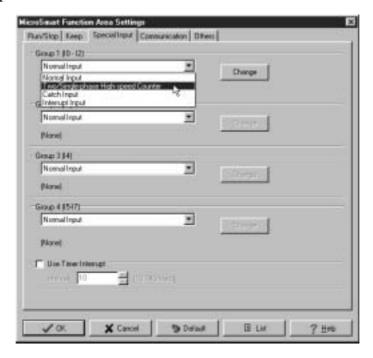
**3.** When using high-speed counter HSC1, select **Two/Single-phase High-speed Counter** in the Group 1 pull-down list box.
