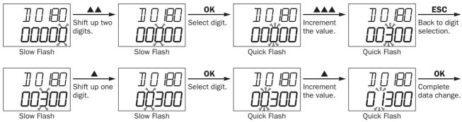
**5.** The changed data is displayed without flashing. Save the changes.
