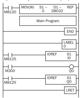
M8120 is the initialize pulse special internal relay.
