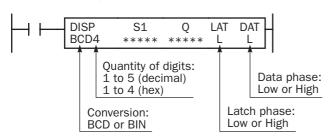
When input is on, data designated by source operand S1 is set to outputs or internal relays designated by operand Q. This instruction is used to output 7-segment data to display units.
