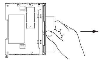
**3.** Do not pull one end of the longer terminal block, otherwise the terminal block may be damaged.
