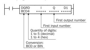
When input is on, data designated by operands I and Q is set to a data register designated by destination operand D1.
