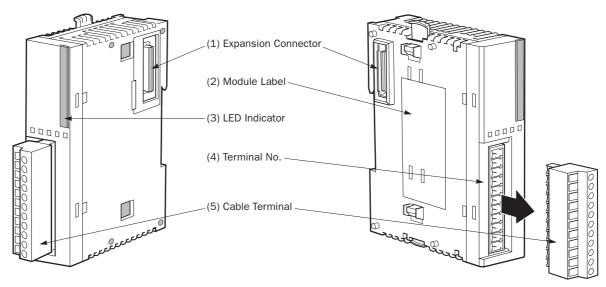
The above figures illustrate the 4-in/4-out mixed I/O module.
