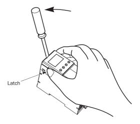
**3.** Remove the HMI module from the HMI base module.
