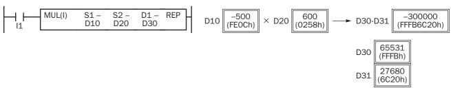
**Note:** Since the destination uses two word operands in the multiplication operation, data register D399 (10-I/O type CPU module) or D1299 (16- and 24-I/O type CPU modules) cannot be used as destination operand D1. When using a bit operand such as internal relay for destination, 32 internal relays are required; so internal relay M281 (10-I/O type CPU module) or M1241 (16- and 24-I/O type CPU modules) or a larger number cannot be used as destination operand D1.
