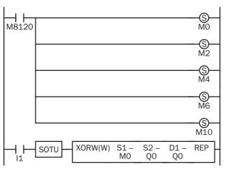
Ten outputs Q0 through Q11 are assigned to 10 internal relays M0 through M11.
