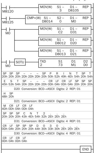
M8120 is the initialize pulse special internal relay.  $3 \rightarrow D8105$  to enable the DSR option for busy control. M8125 is the in-operation output special internal relay. CMP=(W) compares the D8014 second data with 0. When the D8014 data equals 0 second, M0 is turned on.
