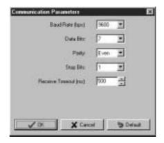
When 2550 ms is selected in the Receive Timeout box, the receive timeout function is disabled.
