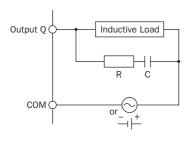
This protection circuit can be used for both AC and DC load power circuits.
