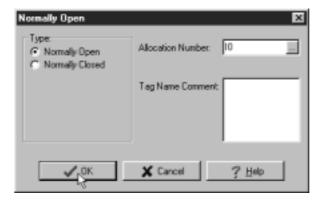
A NO contact of input I0 is programmed in the first column of the first ladder line.
