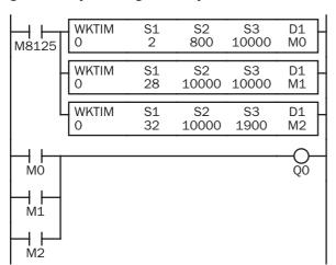
M8125 is the in-operation output special internal relay.
