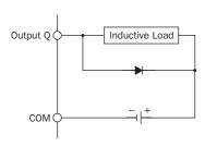
This protection circuit can be used for DC load power circuits.
