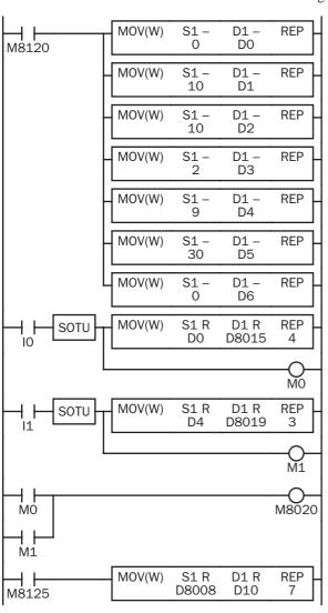
M8120 is the initialize pulse special internal relay.
