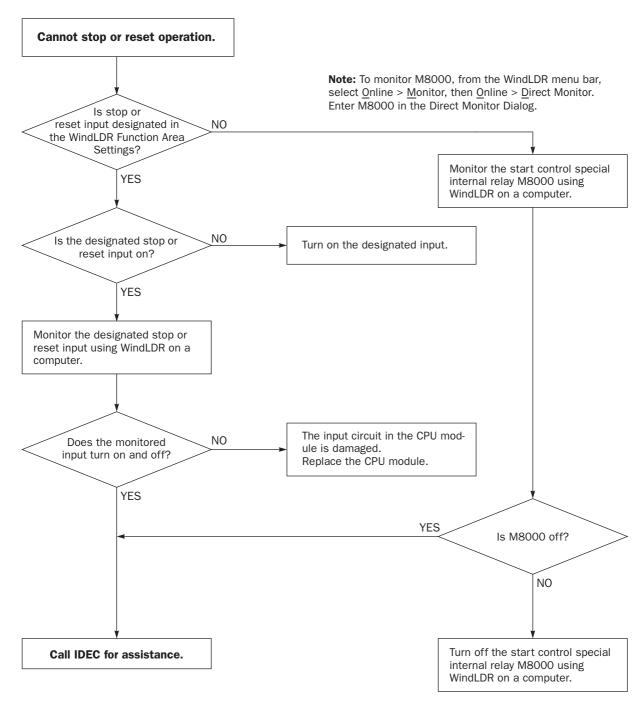
**Note:** To turn off M8000, from the WindLDR menu bar, select  $\underline{O}$ nline >  $\underline{M}$ onitor, then  $\underline{O}$ nline > Direct  $\underline{S}$ et/Reset. Enter M8000 in the Direct Set/Reset Dialog. Click Reset.
