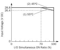
When using at 45°C, all I/Os can be turned on simultaneously at input voltage 28.8V DC as indicated with line (2).
