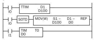
While input IO is on, TTIM measures the ON duration of input IO and stores the measured value in units of 100 msec to data register D100.
