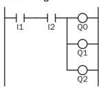
Programming multiple outputs of the same output number is not recommended. However, when doing so, it is good practice to separate the outputs with the JMP/JEND set of instructions, or the MCS/MCR set of instructions. These instructions are detailed later in this chapter.
