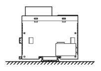
Allowable Mounting Direction at 35°C or below
