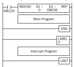
M8120 is the initialize pulse special internal relay.
