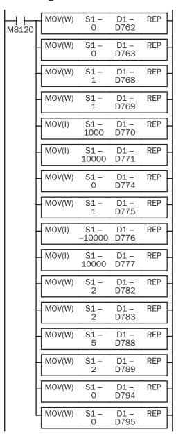
M8120 is the initialize pulse special internal relay.
