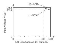
When using at  $45^{\circ}$ C, all I/Os can be turned on simultaneously at input voltage 28.8V DC as indicated with line (2).
