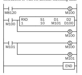
M8120 is the initialize pulse special internal relay used to set M100.
