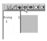
**2.** Move the mouse pointer to the first column of the first line where you want to insert a NO contact, and click the left mouse button.
