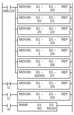
M8120 is the initialize pulse special internal relay.
