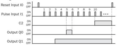
Output Q0 is on when counter C2 current value is 5.
