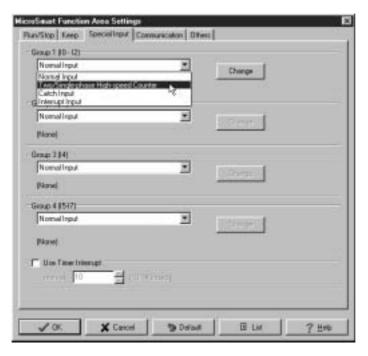
**3.** When using high-speed counter HSC1 or HSC4, select **Two/Single-phase High-speed Counter** in the Group 1 or 4 pull-down list box.
