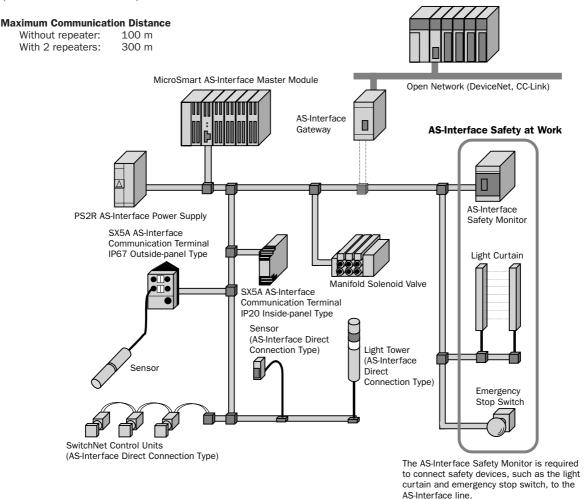
**SwitchNet** <sup>™</sup> SwitchNet is an IDEC trademark for pushbuttons, pilot lights, and other control units capable of direct connection to the AS-Interface. SwitchNet devices are completely compatible with AS-Interface Ver. 2.1.
