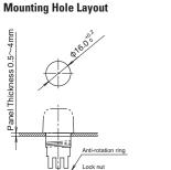
Recommended tightening torque for Locking Ring: 0.29 to 0.49 N-mm.
