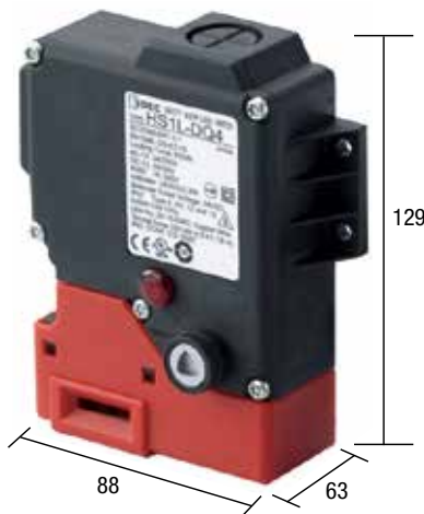
Conventional (HS1L): Volume 715 cm 3 Locking force 3000N
