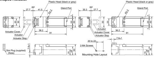
Note: Plug the unused actuator entry slot using the slot plug supplied with the safety interlock switch.
