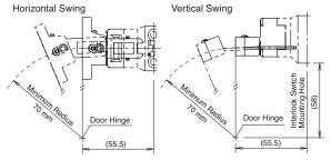
When the door hinge is on the extension line of the actuator mounting surface: 70 mm
