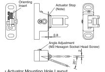
· Actuator Mounting Hole Layout (horizontal/vertical swing) 2-M4 Screw
