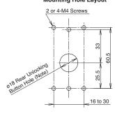
Note: With the mounting hole dimension, the rear unlocking button rod does not touch the hole even when the interlock switch moves sideways.
