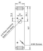
When installing the HS5E-□44L□-G (rear unlocking button type), provide a rear unlocking button hole on the HS9Z-SP51.
