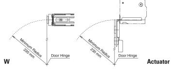
• When door hinge is on the extension line of the interlock switch surface
