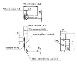
The actuator stop is used to adjust the actuator position. Remove after the actuator position is mounted.
