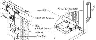
Note: When mounting the actuator, make sure that the actuator enters the slot in the correct direction, as shown on the right
