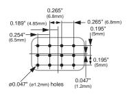
LW□B PC Board Drilling Layout PC Board Terminal Bottom View
