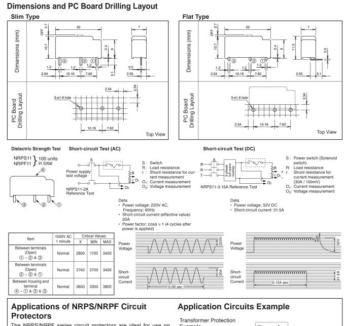
The NRPS/NRPF series circuit protectors are ideal for use on printed-circuit boards in small electric appliances to protect power transformers, rectifiers, small-motors, solenoid valves, and solenoids from overloads.
