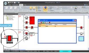
Monitoring a program is possible by connecting PLCs installed in a system. The I/O status can be confirmed on a WindLDR screen. The I/Os of the PLC can be turned on and off in Forced I/O List for testing. Multiple devices can be monitored by using the batch monitor function, increasing the efficiency of debugging
