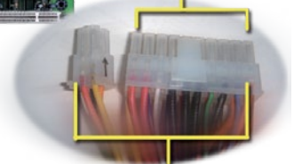
20+4 pin-ATX power connector
