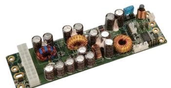
Dedicated ATX power for car PC and battery powered applications
