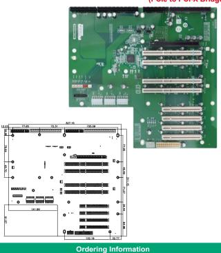
12-slot backplane with one PCIe x16 slot, four PCI-X slots and
