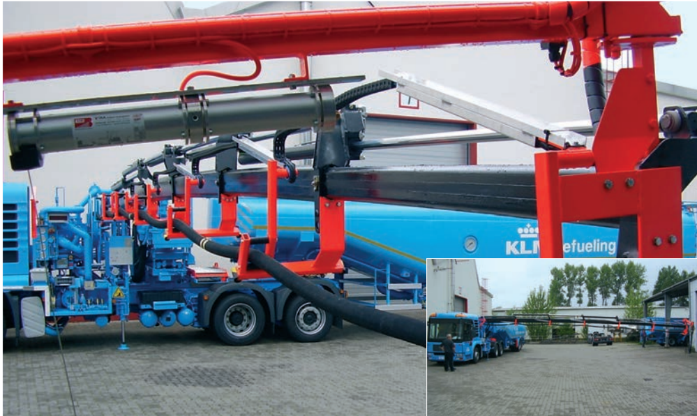
E2/000 series 1400 in aircraft refueling truck - telescopic crane with six sections
