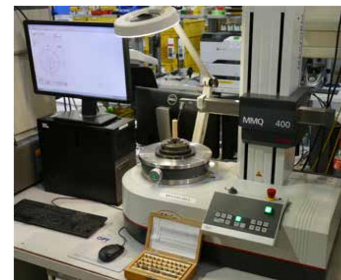
Picture 13: Measurement of the inner diameter of a press-fit plain bearing
