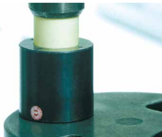
Picture 12: The bearing should be press-fitted using a flat press
