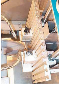
drylin® R linear plain bearings on supported aluminum shafts are used in this grinder to guide the cutting table. The drylin® components stand for extrema dirt resistance, accurate guidance and a smooth operation.
