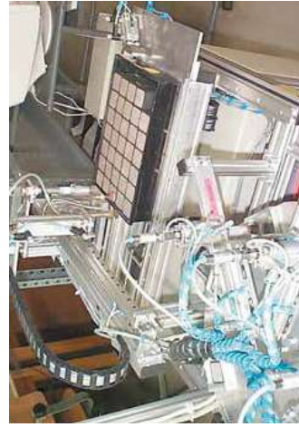
The removal unit is moved along the X-Y axis using the space-saving and cost-saving drylin® N low-profile linear guide. The robust drylin® T guide system undertakes the vertical guidance.
