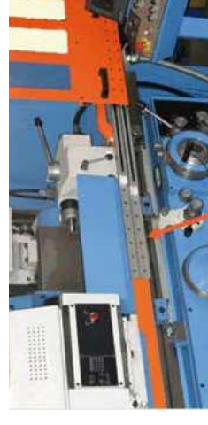
drylin® NT LM in guard door adjustment in a machine tool
