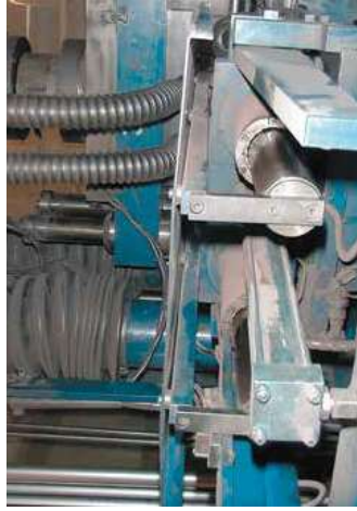
By changing over to the drylin® R linear plain bearing, the maintenance rate of this compaction unit could be extended by two years, despite high stressing from powder particles and abrasive agents.
