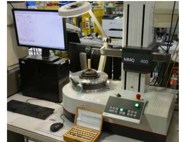
Picture 13: Measurement of the inner diameter of a press-fit plain bearing
