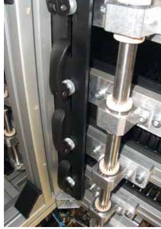
The production line should be adjusted without setup time being required. drylin® linear guides, which enable precise and fast adjustment, were used for this.
