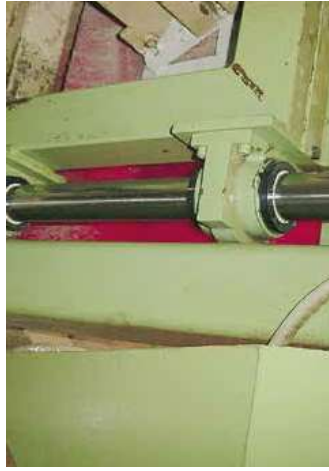
The machine now runs entirely free of troubles for multiple years with drylin® R/JUM-01 linear bearings despite the extremely heavy – duty operation.
