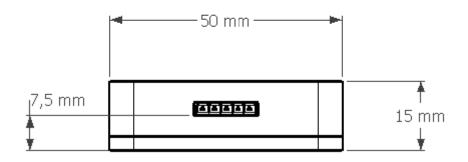
Figure 4: SQ device dimensions (mm)
