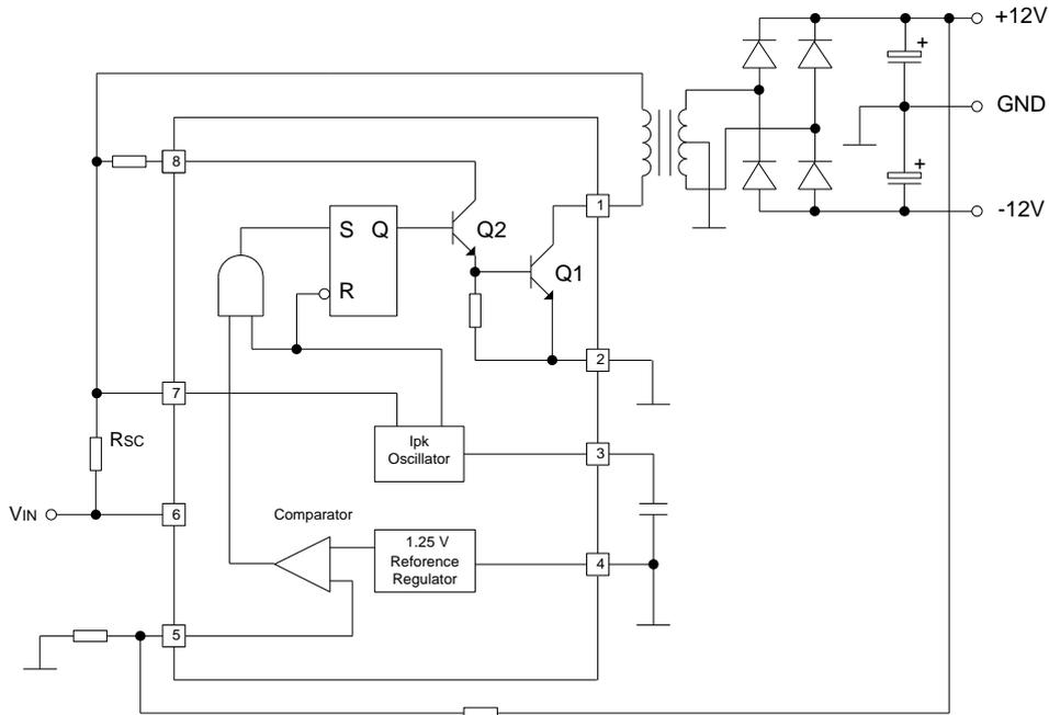
Higher Output Power, Higher Input Voltage
