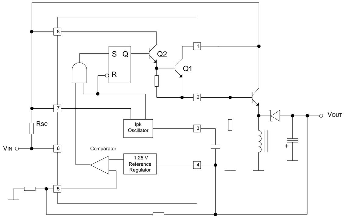
Voltage Inverting With External PNP Saturated Switch
