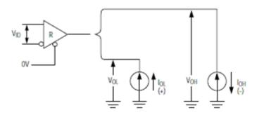
Figure 3. Receiver  $V_{\text{OH}}$  and  $V_{\text{OL}}$
