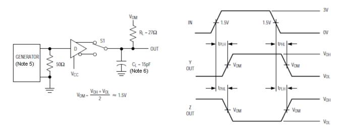
Figure 5. Driver Propagation Times
