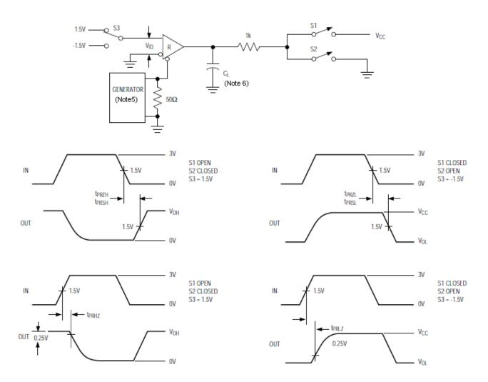
Figure 9. Receiver Enable and Disable Times
