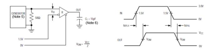
Figure 8. Receiver Propagation Delay
