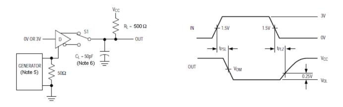
Figure 7. Driver Enable and Disable Times ( $t_{\text{PZL}},\,t_{\text{PSL}},\,t_{\text{PLZ}}$ )
