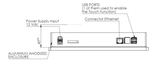
Ethernet and USB port connectors (One of the USB ports is connected in order to activate the attach function)
