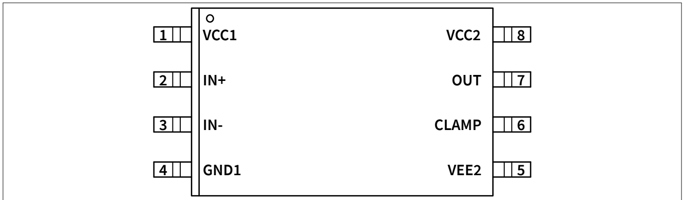
Figure 5 PG-DSO-8 (top view)
