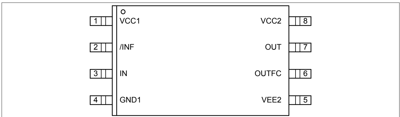
Figure 4 Pinout clamp configuration (top view)
