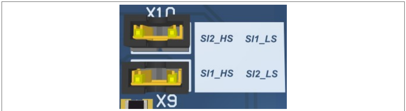
Figure 17 SI1, SI2 jumper cross-connect placement
