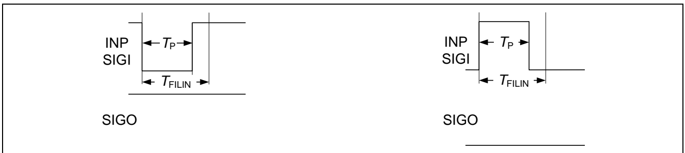
Figure 9 Timing of short pulse suppression terminal INP and SIGI ( T_P < T_{FILIN} )
