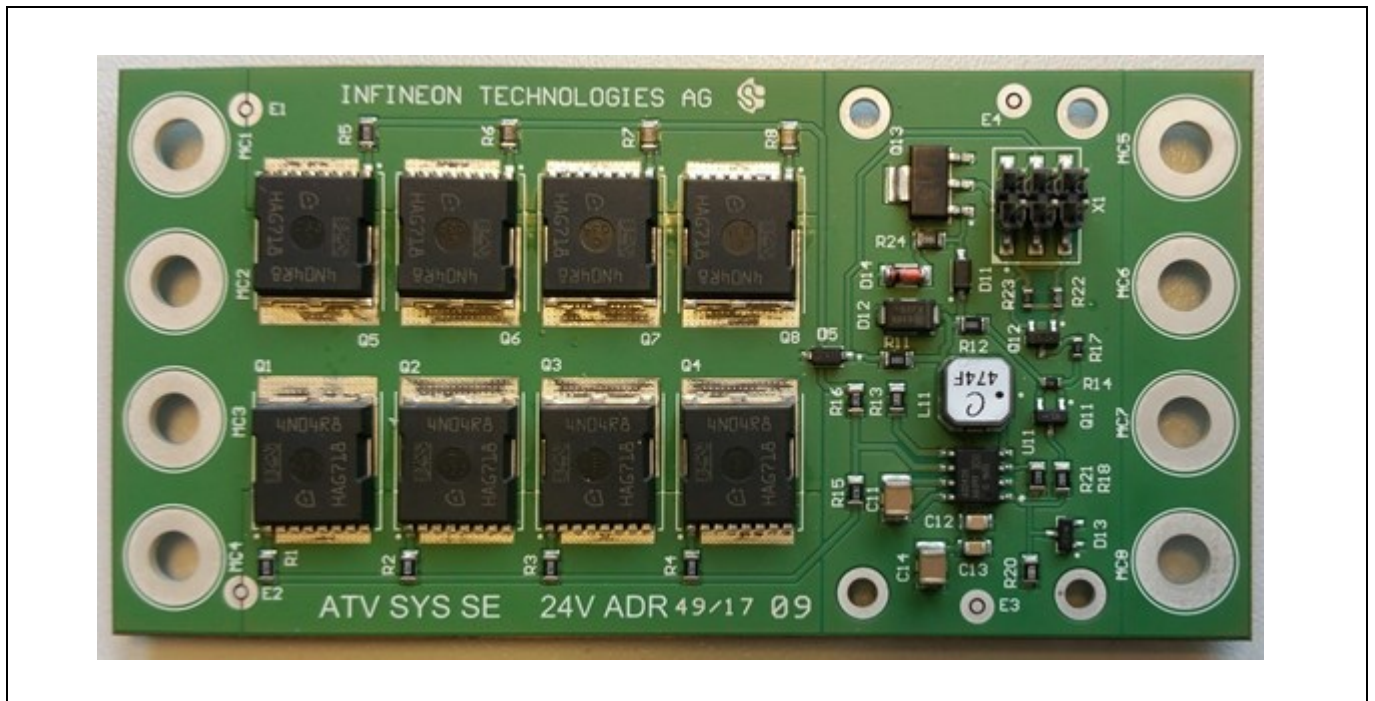
Figure 2 Battery Switch 24V - System Demonstrator Top View
