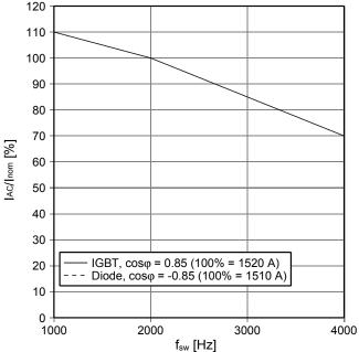
$$\begin{split} &T_{\text{inlet}} \text{- derating curve IGBT (motor), Diode (generator)} \\ &V_{\text{DC}} = 1100 \text{ V}, \text{ V}_{\text{AC}} = 690 \text{ V}_{\text{RMS}}, f_{\text{sw}} = 2 \text{ kHz, } f_{\text{AC sine}} = 50 \text{ Hz,} \\ &cos\phi = \pm 0.85 \text{ and nom. cooling conditions} \end{split}$$
