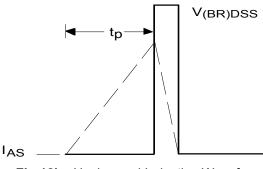
Fig 12b. Unclamped Inductive Waveforms
