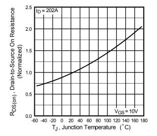
Fig. 4 Normalized On-Resistance vs. Temperature
