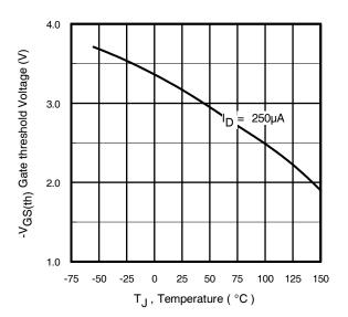
Fig 14. Threshold Voltage vs. Temperature
