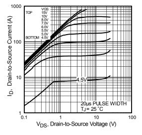
Fig. 1 Typical Output Characteristics
