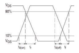
Fig 10b. Switching Time Waveforms
