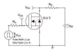
Fig 18a. Switching Time Test Circuit
