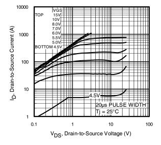
Fig. 1 Typical Output Characteristics
