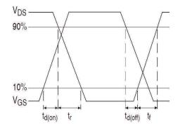
Fig 18b. Switching Time Waveforms
