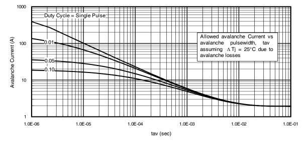
Fig 15. Typical Avalanche Current vs. Pulse width
