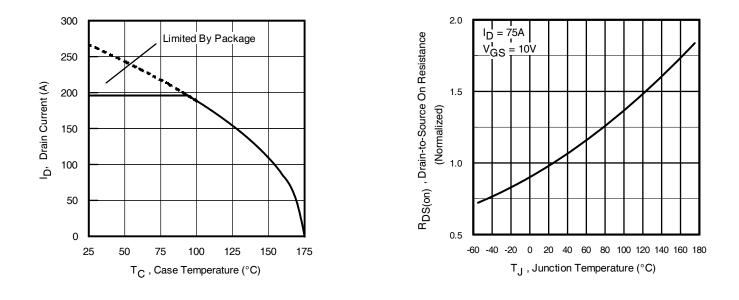
Fig 9. Maximum Drain Current vs. Case Temperature
