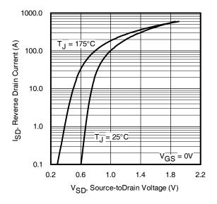
Fig. 7 Typical Source-to-Drain Diode Forward Voltage
