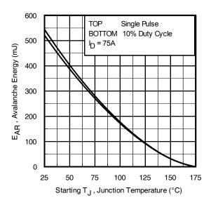
Fig 16. Maximum Avalanche Energy vs. Temperature
