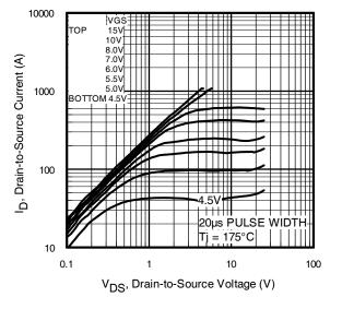
Fig. 2 Typical Output Characteristics
