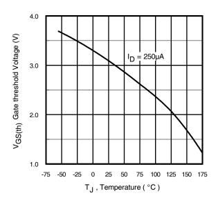
Fig 14. Threshold Voltage vs. Temperature
