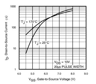
Fig. 3 Typical Transfer Characteristics
