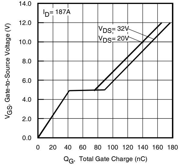
Fig 6. Typical Gate Charge vs. Gate-to-Source Voltage
