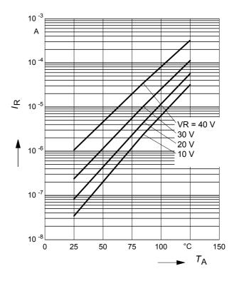
**Reverse current**  $I_{R} = f(V_{R})$  $T_{A}$  = Parameter (per diode)
